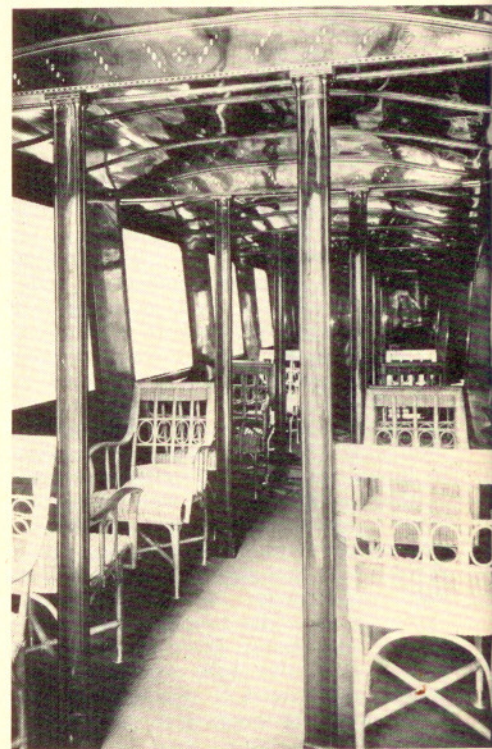
The inside of the 24-passenger cabin of Deutschland shows the lightweight wicker chairs and ornate woodwork. Hot meals could be served in flight.
